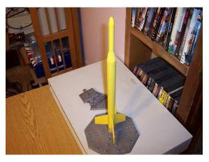
Below is the **Estes Screamin' Mimi**. This kit is parachute recovery, which I plan to launch on a D12-5 motor.
